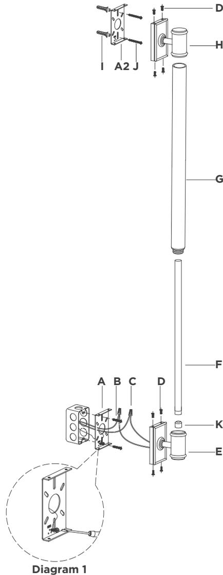
11. Remove protective caps (**K**) from fixture (**E**), then install light source (**F**) to fixture (**E**).
